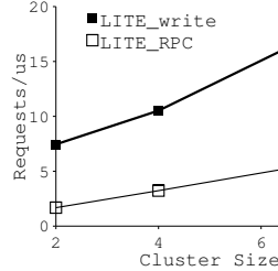
Figure 14: Scalability of LITE RDMA and RPC. Each node runs 8 threads. LT_write writes 64B. LT_RPC sends 64B and gets 8B reply.
